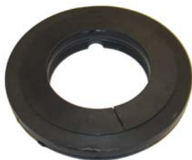
Failed Seal Resulting from Improper Fit
