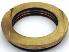
Failed Seal Resulting from Improper Installation
